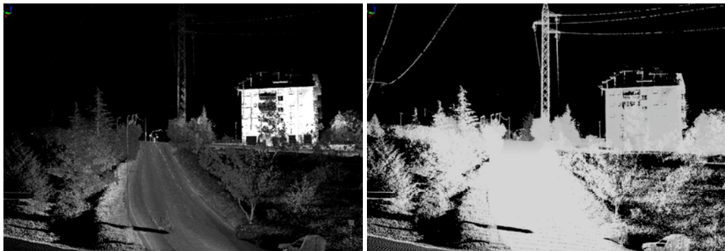
Figure 7. A point cloud represented with and without intensity data to evidence the coverage of observed area in both horizontal and vertical directions. The prospective view shows also the high-voltage electric lines.
