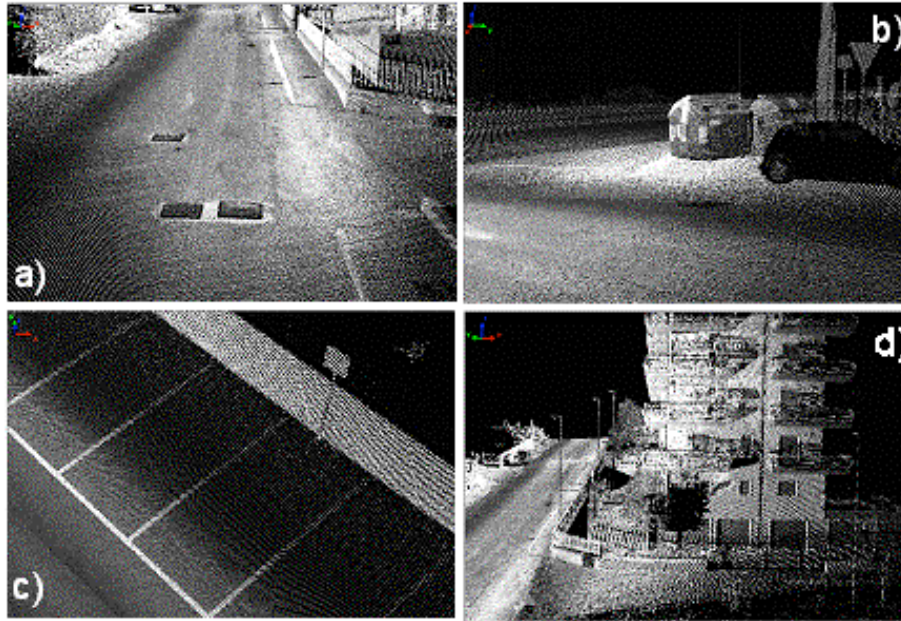
Figure 6. Point cloud details. a) Drain covers in the street, b) pillars, road signs and dustbins, c) parking lines and d) architectural features are well determined and measured at centimetre level accuracy.
