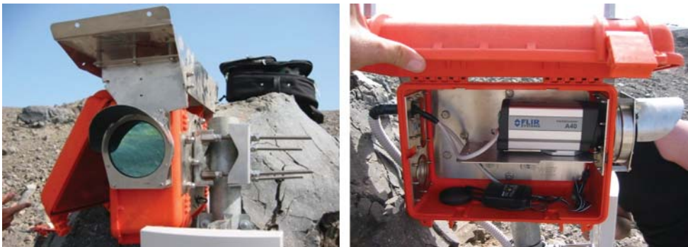
Fig. 5. Polycarbonate box containing the A 40 M FLIR thermal camera.
