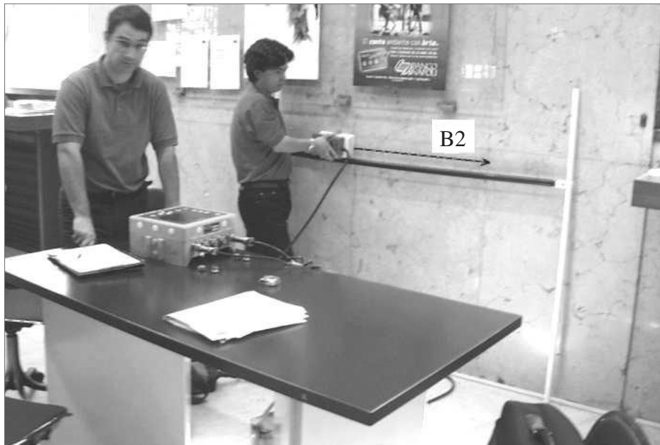
Fig. 6. Photo of the travertine panel inside to the Bank of Naples in Campobasso with the location of B2 radar profile.
