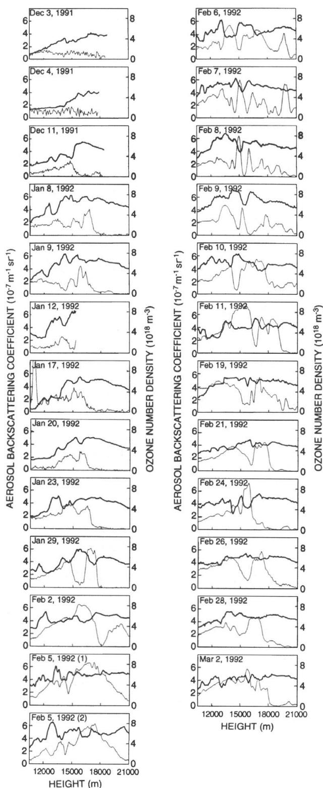
**Fig. 4.** Sequence of vertical profiles of aerosol backscattering (thin line) and ozone number density (heavy line), observed with lidar at Thule from December 3, 1991 to March 2, 1992 (di Sarra *et al.*, 1992).
