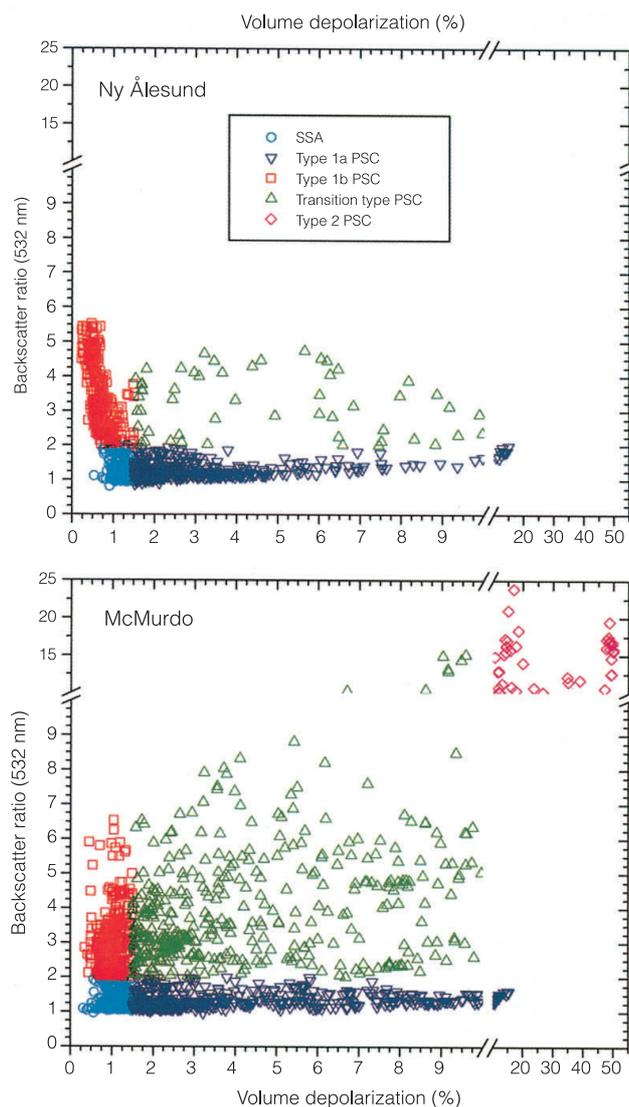
**Fig. 3.** Scatter plot of 532 nm backscatter ratio versus volume depolarisation from lidar measurements at Ny Ålesund, Spitsbergen (upper panel) and Antarctic measurements at McMurdo (lower panel), illustrating the grouping of different particle types observed in the polar winter stratosphere (adapted from World Meteorological Organization, 1999, courtesy R. Neuber and A. Adriani).
