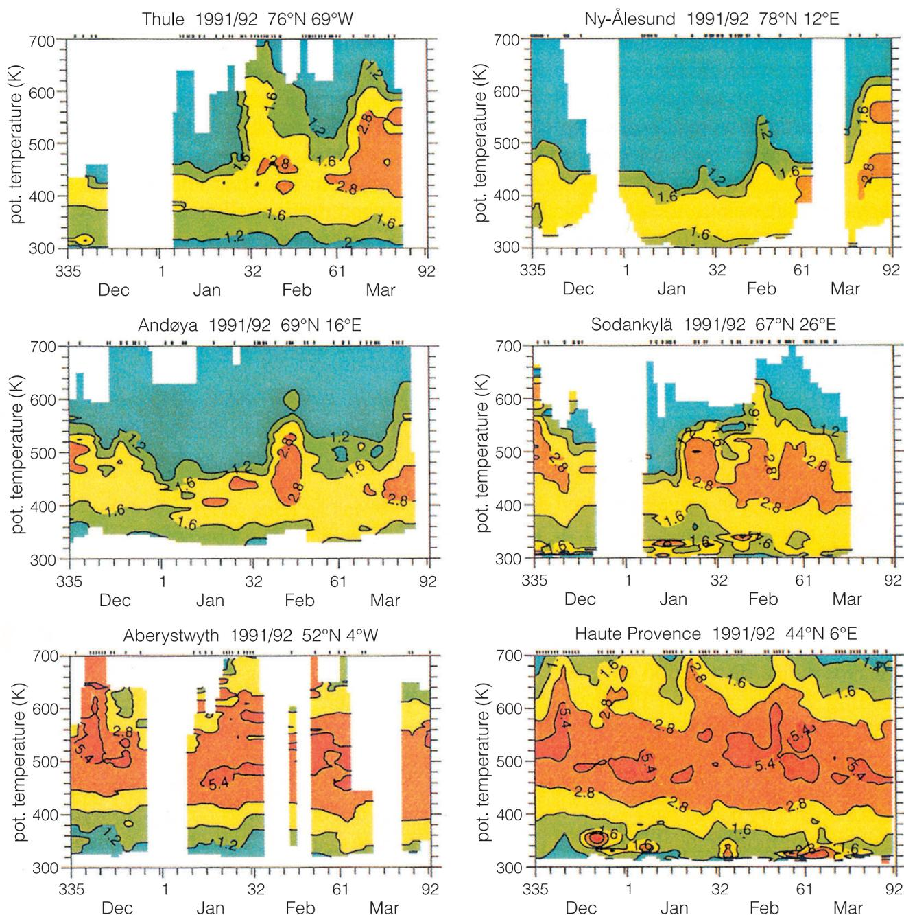
**Fig. 7.** Temporal development of the backscatter ratios at six lidar stations in the period December 1991 through March 1992 during EASOE (European Arctic Stratospheric Ozone Experiment). The bars above the plots indicate times of the measurements. Isolines are set to values of 1.2, 1.6, 2.8, and 5.4 in order to reveal greater details for the lower values. Adapted from Neuber *et al.* (1994) (copyright by the American Geophysical Union).
