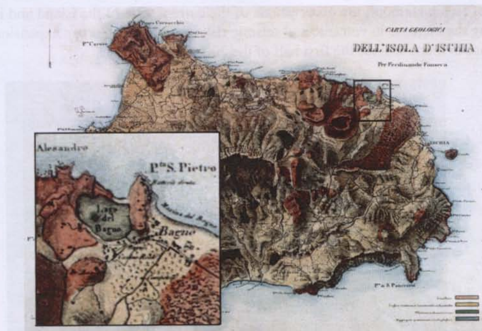
Fig.2 - First geological map of Ischia produced by Fonseca (1847), scale 1:25,000. The most recent lava flow and lava and scoria cones are represented in red-brown. Inset with a close-up of the Lago del Bagno zone.
