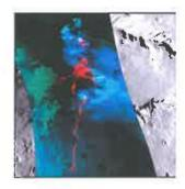
True-colour image acquired by airborne MIVIS (Mt. Etna July 2001) and draped over a 10 m resolution shaded relief. High spatial and radiometric resolution provides high quality estimation of effusion rates.
