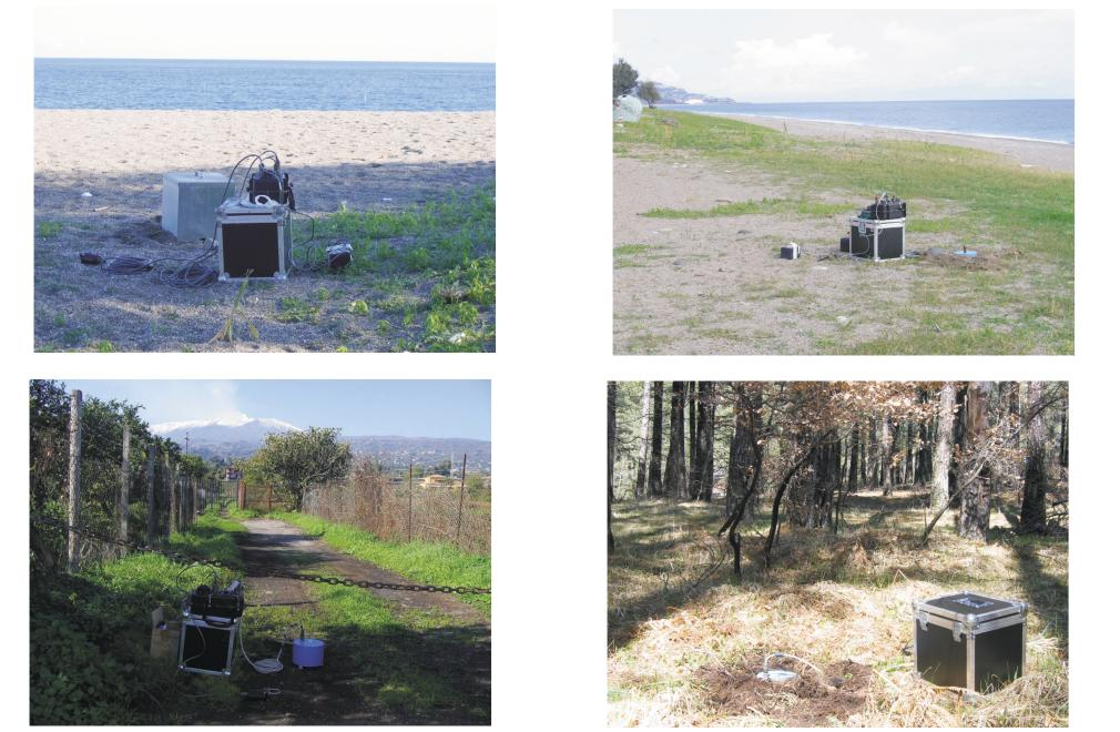
Pictures showing some sites of seismic noise recordings along the Pernicana fault system. We used Lennartz Le3D-5s sensors with Reftek R130 digitizers.
