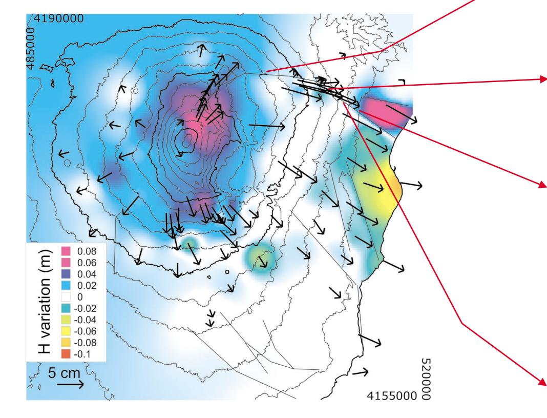
**Displacement vectors** and height variations from the comparison between July 2005 and June 2006. The arrows represent the horizontal displacement vectors, while the vertical displacement is shown by a colour map obtained by interpolating the measurements relevant to each benchmark (redrawn from Bonforte et al., 2008).
