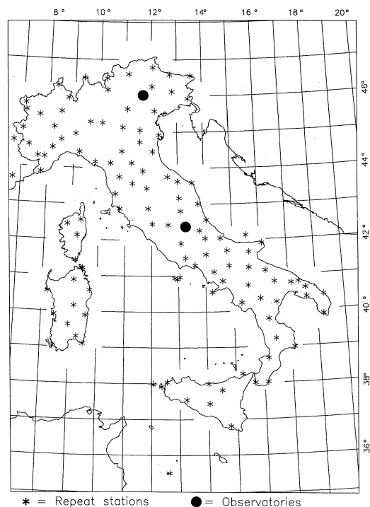
Fig. 1. Italian repeat stations network at 1990.0. Filled circles indicate observatories (L'Aquila 42.38°N, 13.32°E; C. Tesino 46.05°N, 11.65°E).
