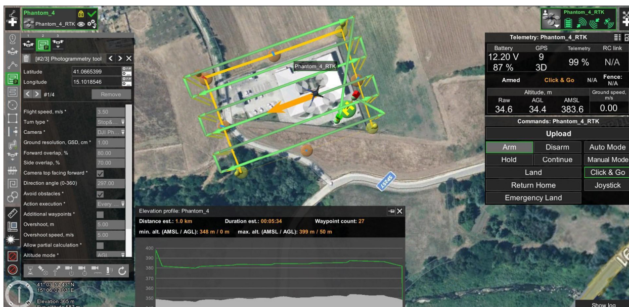
Figure 6. UgCS Enterprise v. 4.20 software interface for UAS mission planning. In the left panel are shown the set parameters for the flight plan; the right panel shows the UAS telemetry, and the bottom window displays the survey’s altimetry and number of waypoints.
