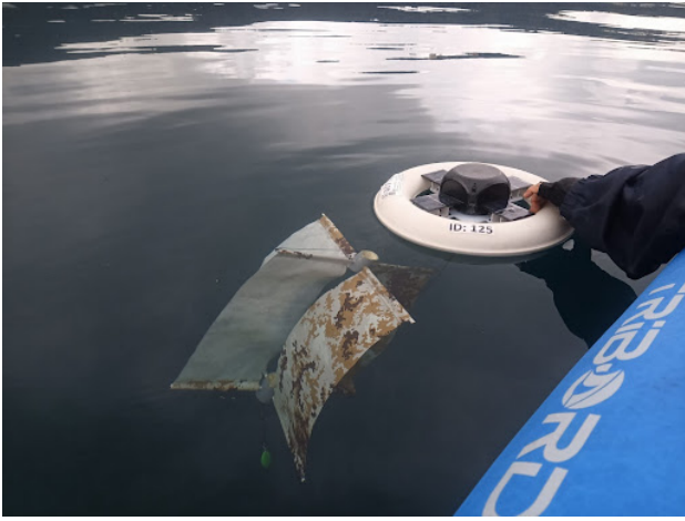
Fig. 2. Low-cost CARTHE-like drifter used in Lago Albano.
