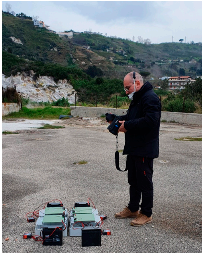
Figure 3. Positioning of DTTs during a survey. The grey box allows the transport of each of the single targets assembled.
