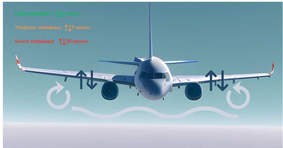
Figure 3. Schematic illustration of the role of the jet stream and velocity shears in driving aircraft turbulence. Green, orange, and red texts report the three different categories of aircraft turbulence together with the expected bumpiness in meters.
