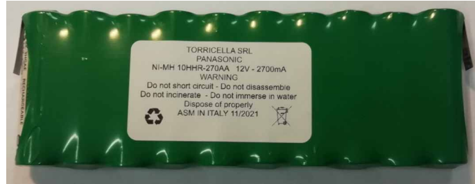
Figure 7 Image of 12V NI-MH battery pack placed inside the Junction Box.
