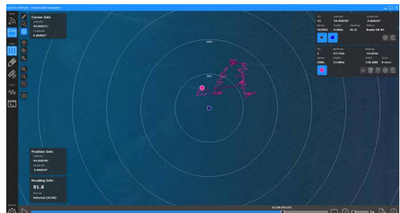
Figure 12 Example of visualization of the USBL tracking by using Seatrac PinPoint software; purple line identifies the track of submarine target. The upper right panel gives information about the position of the Vessel and USBL target.
