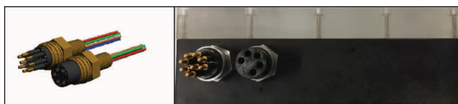
Figure 6 Details of the two marine connectors: left panel, CAD representation; right panel, real view.
