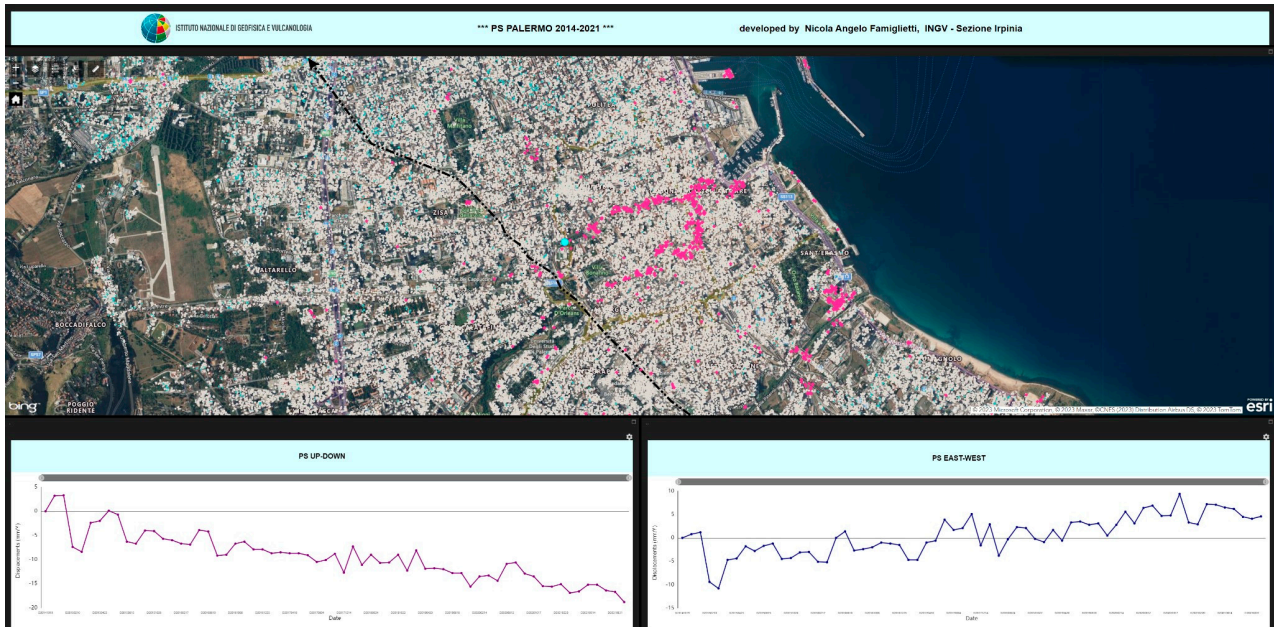
Figure 9. PSs Palermo WebApp implemented by authors of this work using ArcGIS online suite. The points in the map are the PS on the E-W and Vertical components. The Two graphs show the time series of the selected PS in the map.
