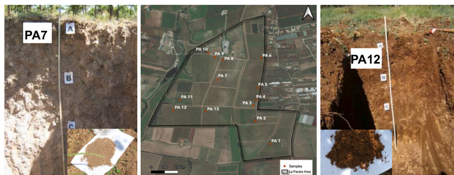
Fig. 3. Profiles and field aspect of the two types of soils in the investigated area. Most diffuse, brown and clayey soils (right) and gray and sandy soils (left) are shown. Location of sampling sites is shown in the photo in the center. Samples for laboratory analyses were collected at about 40 cm of depth. (For interpretation of the references to colour in this figure legend, the reader is referred to the Web version of this article.)
