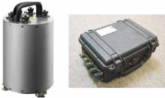
Figure 5 The 40TD broadband Guralp seismometer on the left and the DCM/EAM Guralp acquisition module on the right.
