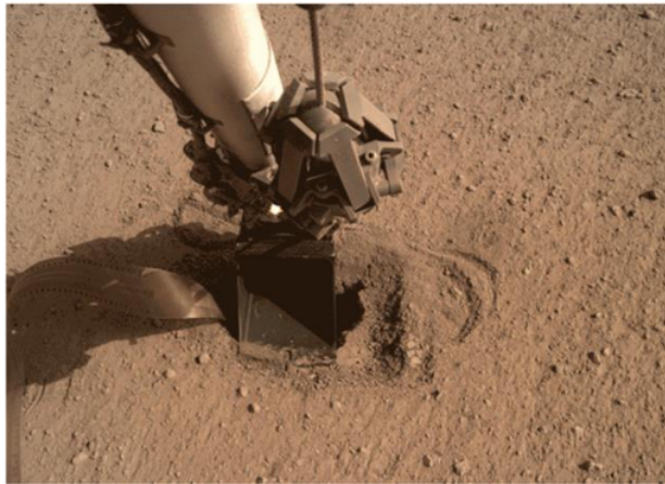
85 86 Figure 2. IDC photo showing the scoop of the Instrument Deployment Arm compressing the regolith 87 above a hole developed around the self-penetrating mole during hammering. The scoop width is 88 7.6 cm (image credit NASA – CalTech).
