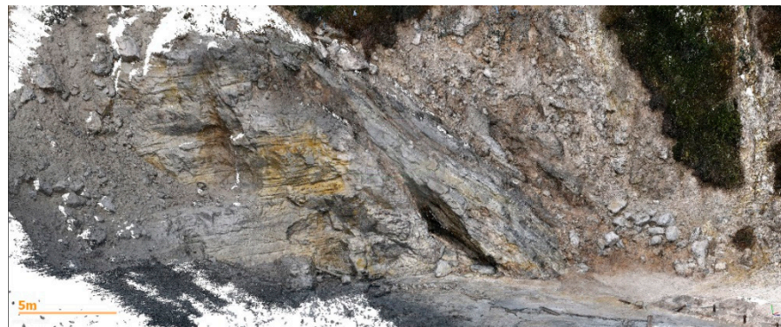
Figure 2. Overview of the point cloud, with RGB color, of the fault L1 object of this study. The image shows the good quality of geomatic data at the main surface and across the L1 fault (compare with Figure 1b). The orange scale bar is 5 m.
