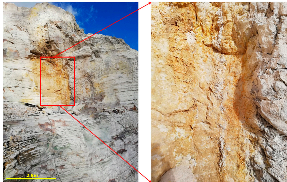
Figure 15. Image (net loss area in Paleo–Astroni deposits, Figure 1c) showing the structural lineament within the Paleo–Astroni deposits filled by alunite, mascagnite, alunogen, alum(K), and amorphous.
