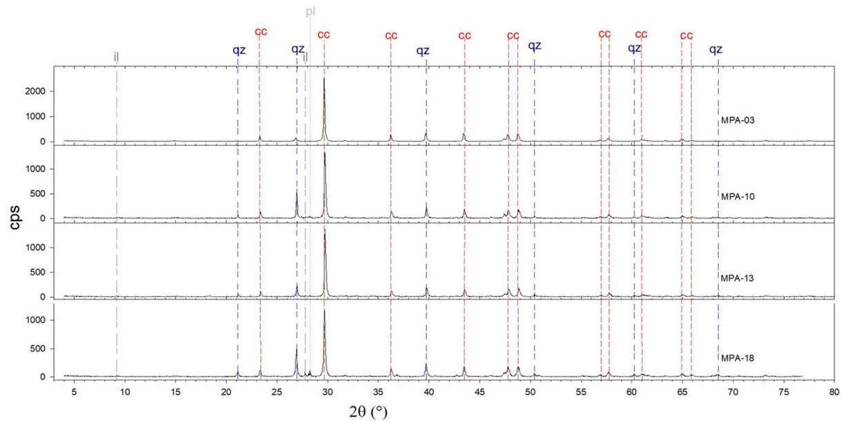
Fig. S3a. Stacked XRPD patterns of concrete ([Table 1S](#)); the vertical lines correspond to Bragg reflections of crystalline standards of the ICSD database; cps indicates count per second; calcite (cc), quartz (qz), illite (il), plagioclase (pl).
