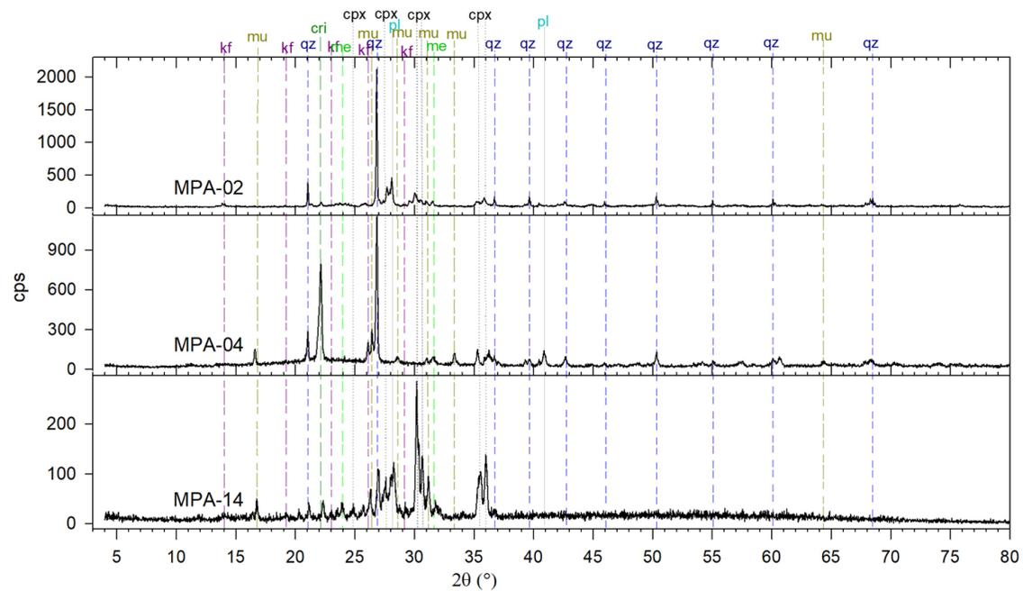
Fig. S3c. Stacked XRPD patterns of bricks (Table 1S); the vertical lines correspond to Bragg reflections of crystalline standards of the ICSD database; cps indicates count per second; calcite (cc), quartz (qz), plagioclase (pl), cristobalite (cri), k-feldspar (kf), clinopyroxene (cpx), mullite (mu), melilite (me).
