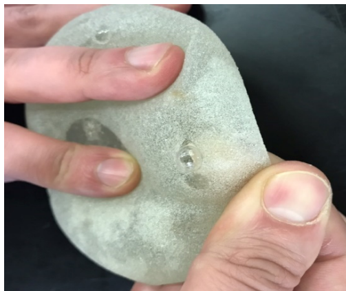
Figure 5: Damage of the prosthesis and gel leakage after impact.
