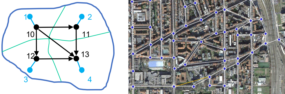
Figure 4: On the left example of four-zone zoning and representation of the transportation network consisting of links and nodes; on the right real example of representation of the transportation network consisting of links and nodes.
