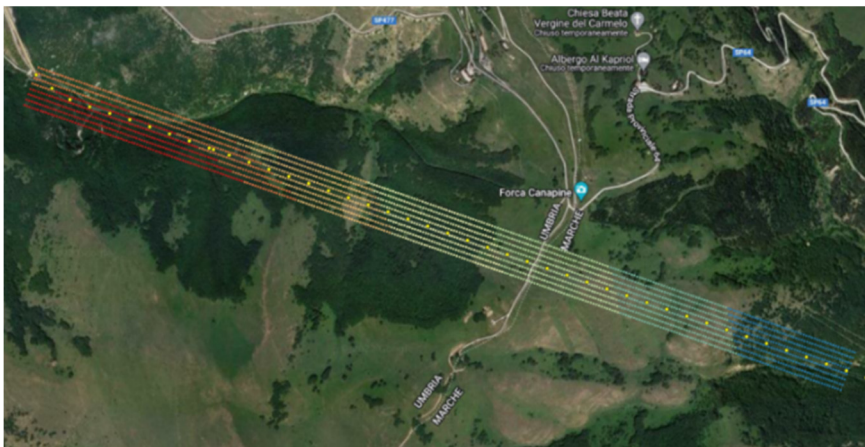
Figure 5: Geostatistical estimate of the vertical acceleration peak in the nodes of the 3D grid 13.5 m in the direction of the longitudinal axis of the San Benedetto tunnel (yellow dots) and 27.0 m in the transverse vertical plane.
