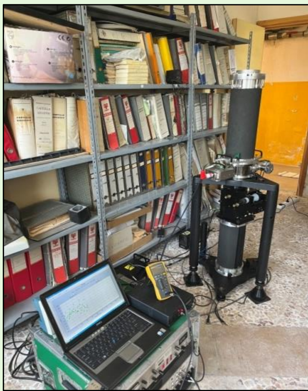
Fig. 2 Measurements with FG5#238 at CNT absolute station.
