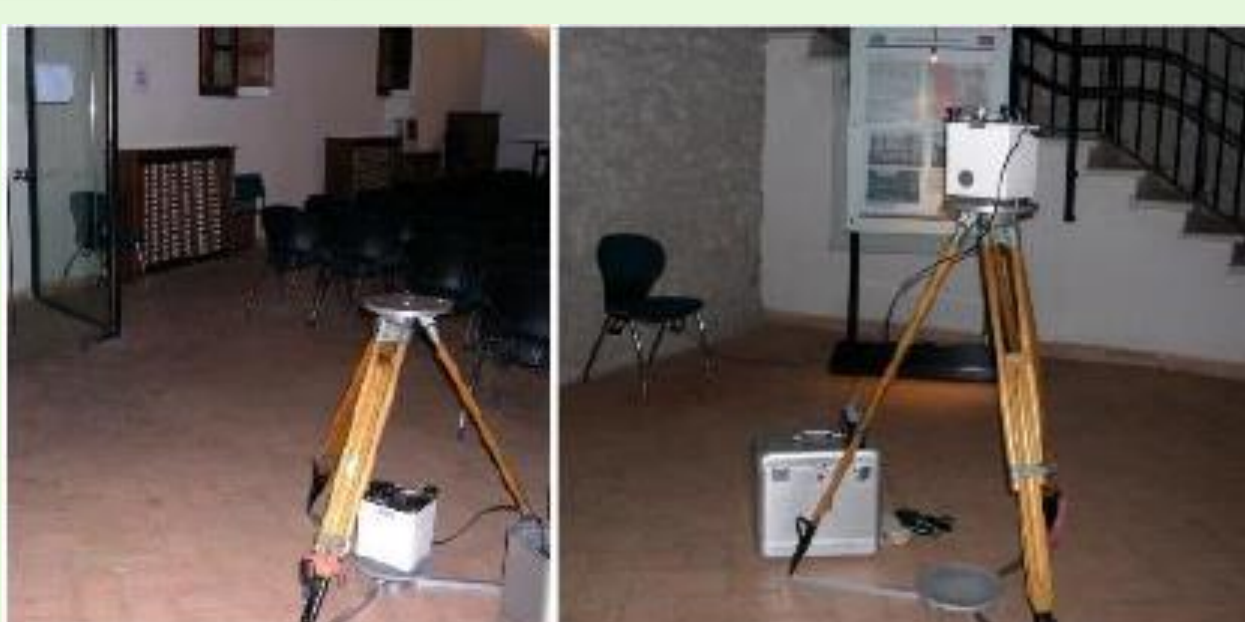
Gravity gradient measurements with LCR D85
