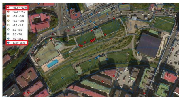
Figure 26 - COSMO-SkyMed persistent scatterers along ascending orbit acquired in the same time span of the topographic monitoring taken (mm/year) (Credits UniNa - DISTAR)
