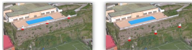
Figure 25 - Location of the monitored points, on the top and at the foot of the embankments (Credits UniNa - DISTAR)
