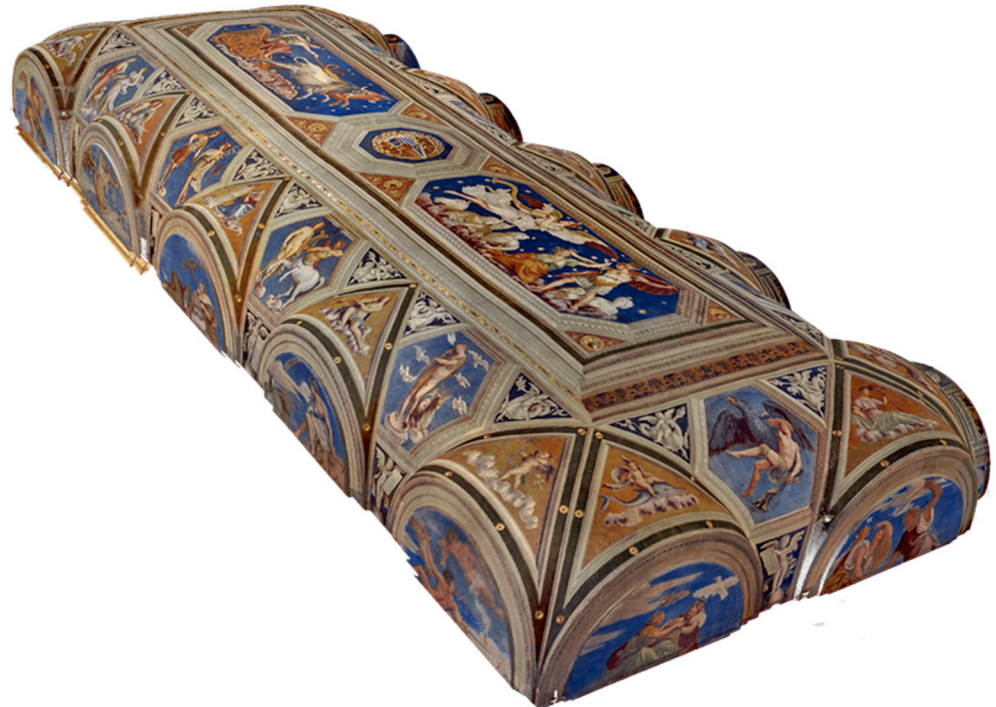
Figure 3. 3D reconstruction of the Lodge of Galatea through the alignment of six point clouds.
