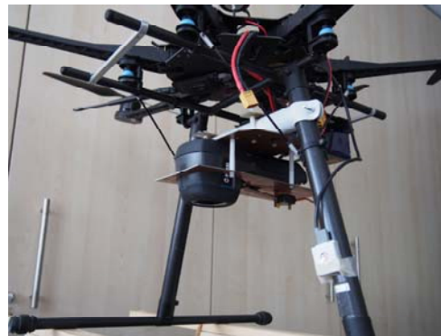
Fig. 7 The thermal camera connected to the UAV
