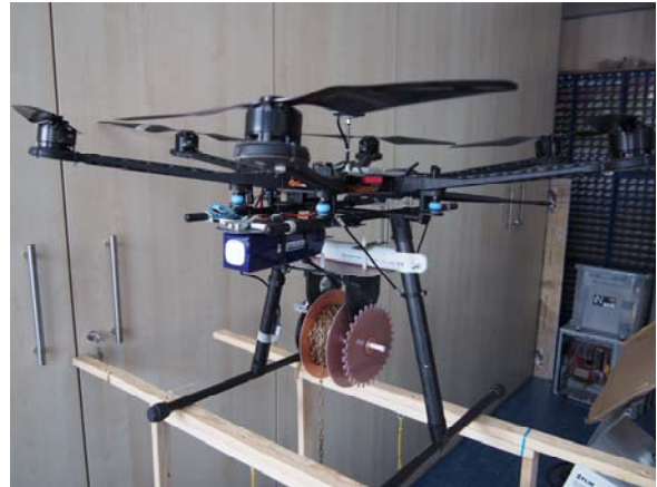
Fig. 3 The winch connected to the UAV
