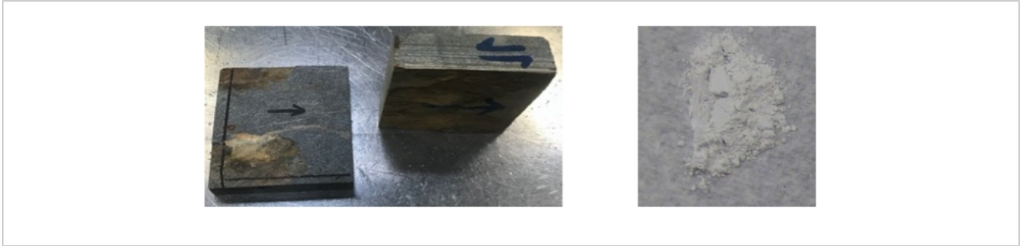
Figure 1: Representative images of the tested fault rocks: solid foliated vs. powdered material. (left) Solid foliated samples sheared parallel to the natural foliation marked by the arrows. (right) Powders obtained by crushing and sieving the solid foliated rock. Please click here to view a larger version of this figure.
