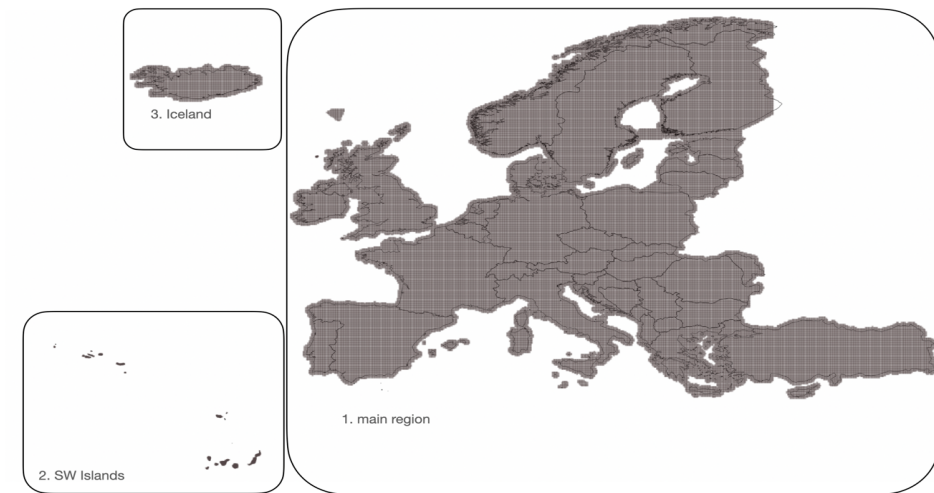
Fig. 5.3 Computational grid for seismic hazard calculation of ESHM20 – the grid points are equally spaced at 0.1 to 0.1 degrees – total number of grid points 97920.
