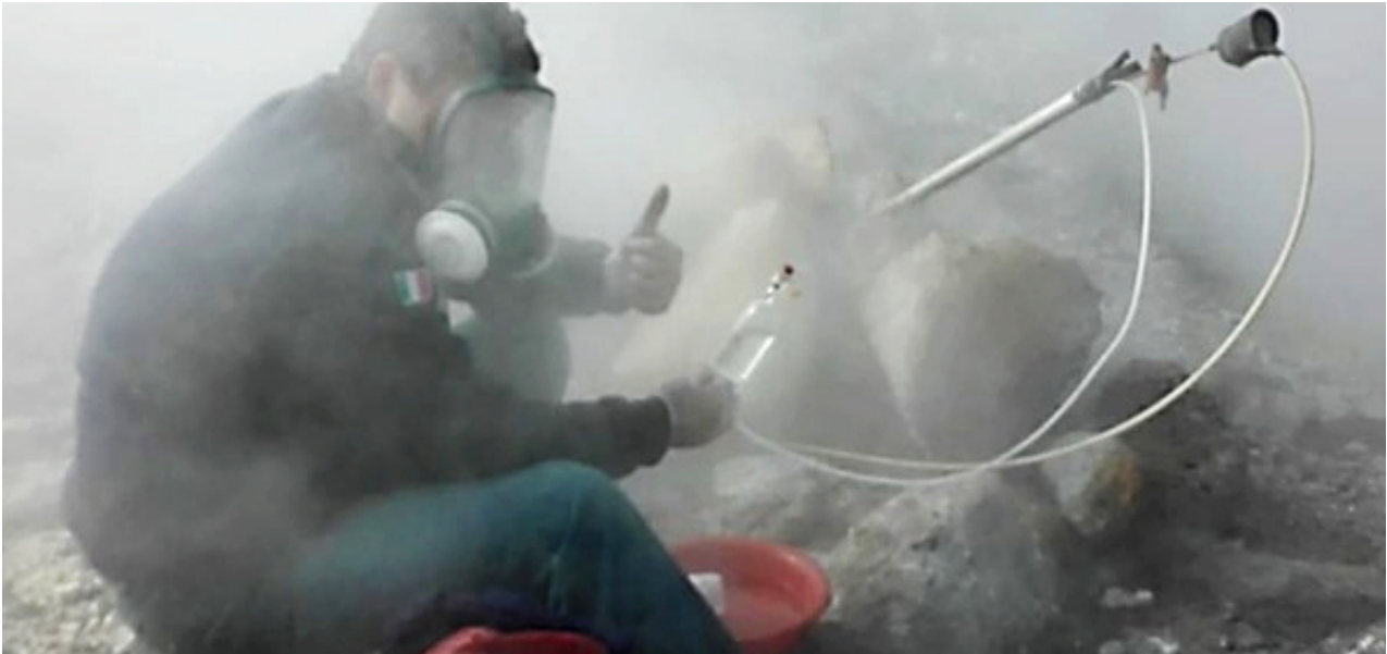
Figure 11. Sampling of fumaroles at Pisciarelli, in the Campi Flegrei Caldera. Source: Photograph by Emanuela Bagnato.
