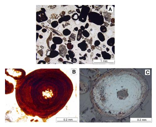
**Figure 5.** Terrestrial iron spherules from Panarea (Aeolian Archipelago, Mediterranean Sea). The newly formed ooids are associated to a hydrothermal origin. (**A**) Transmitted-light photomicrograph of thin-sectioned material illustrating main ooidal morphologies. (**B**) Transmitted- and (**C**) reflected-light photomicrographs of a thin-sectioned ooid with goethite lamination around an indistinct nucleus. Photos B and C courtesy of F. Messori.
