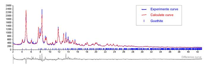
Figure 4. Synchrotron X-ray powder diffractometric pattern of Panarea ooids. The unique Fe-rich mineral identified is goethite.
