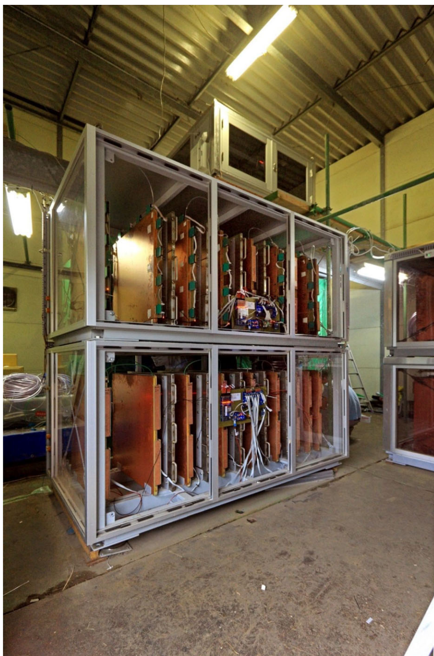
Figure 2. Photograph of three multi-wire proportional chamber-based muography observation system (MMOS) [40]. Eleven MMOS operated in the Sakurajima Muography Observatory during 2021. The MMOS covers a surface of 8.25 m 2 . (Online version in colour.)
