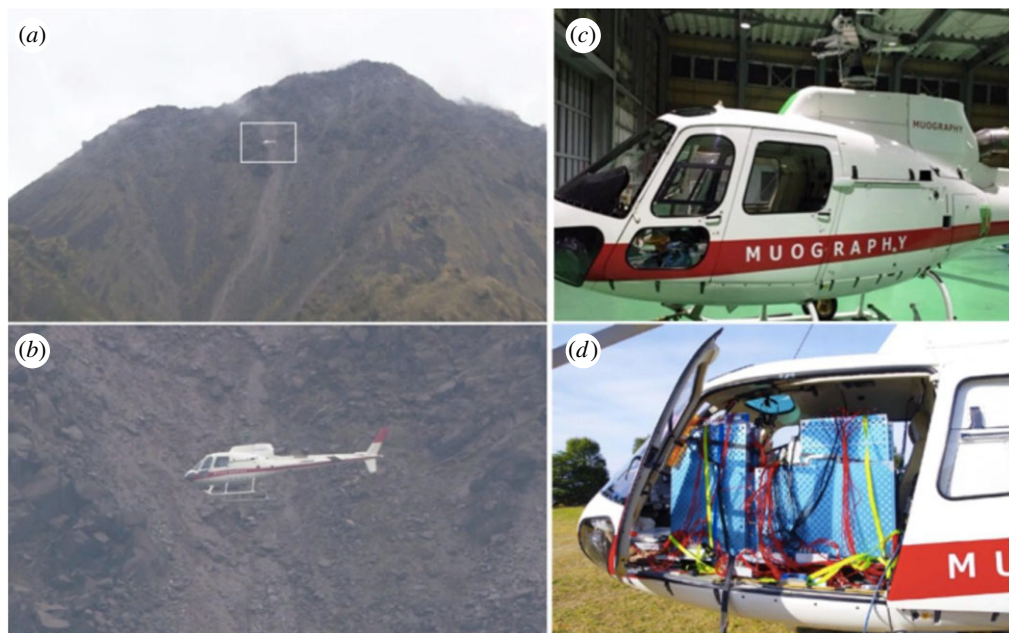
Figure 1. Airborne muography observations at Unzen volcano, Japan [39]. (a) Panoramic view of the volcano with the position of the helicopter carrying the instrument, the white rectangle indicates the position of the helicopter; (b) blow-up image of the helicopter seen in (a); (c) helicopter without instrument; (d) helicopter loaded with the instrument. (Online version in colour.)
