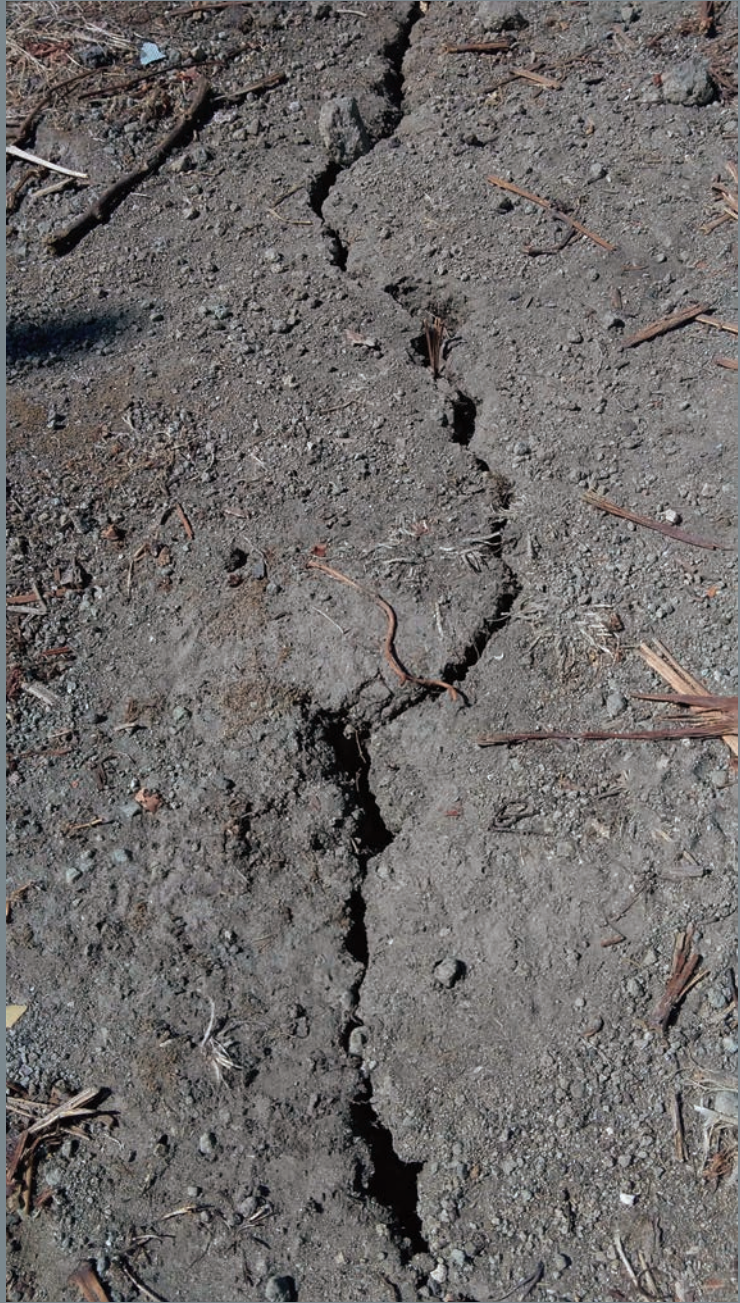
Photo 6 (40.741751° 13.886823°) Coseismic rupture in the soil in the driveway of the same private property of photo 4 (Via Crateca, Fango).
