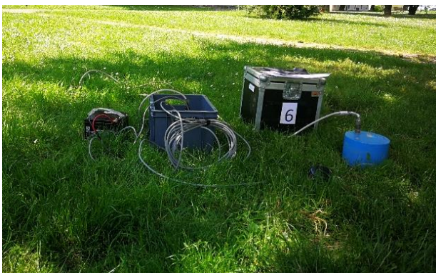
Figure 7: Left: Single station ambient noise measurement. Right: 2D passive ambient noise array installed close to the IT.BRSA accelerometric station.
