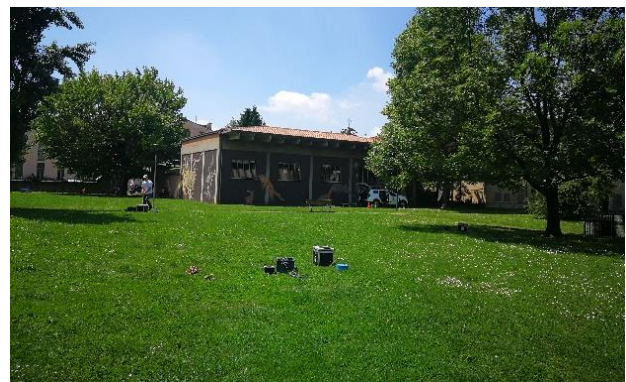
Figure 7: Left: Single station ambient noise measurement. Right: 2D passive ambient noise array installed close to the IT.BRSA accelerometric station.
