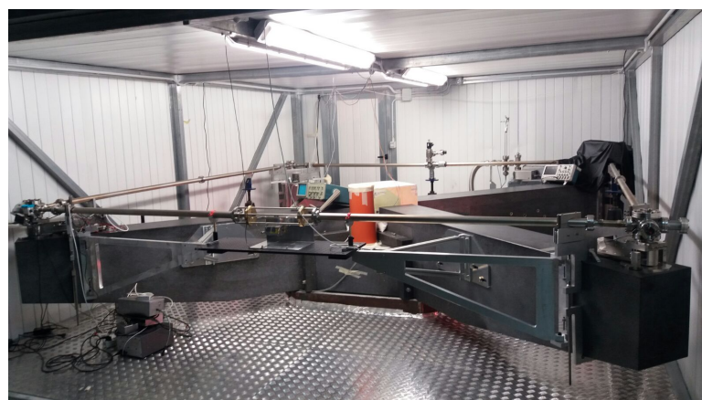
Figure 1. The Gingerino active ring laser gyroscope inside the Gran Sasso national laboratory of the INFN.
