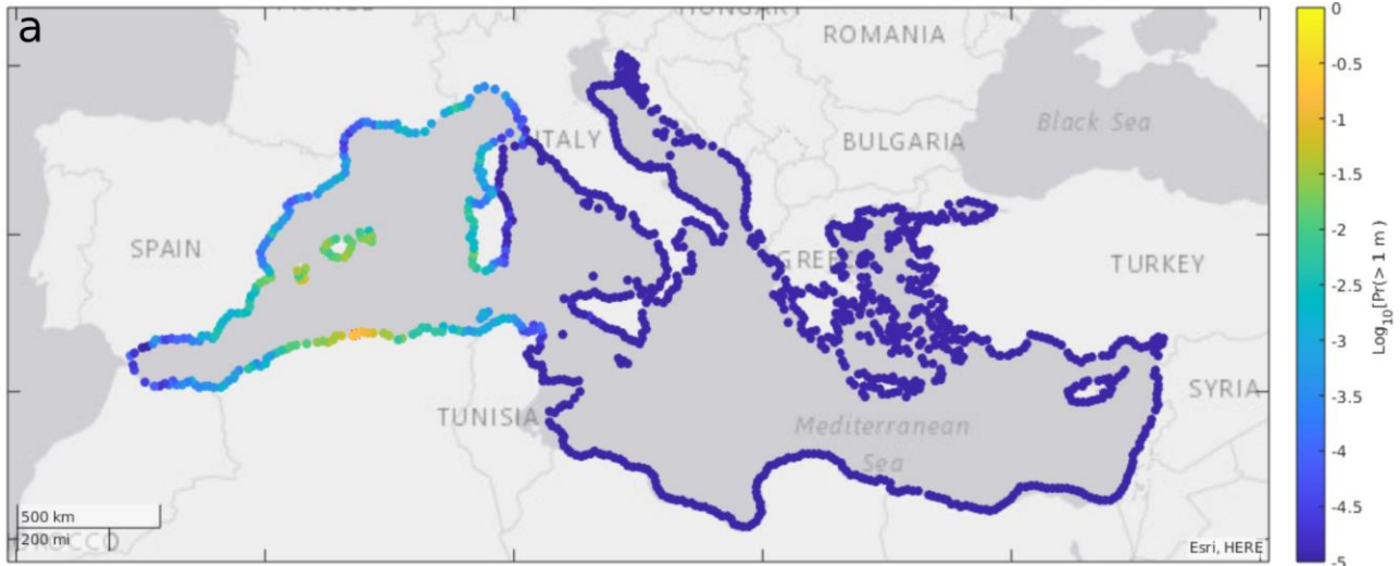
2748 Figure 6: a) Example of PTF results for the Zemmouri-Boumerdes M6.8 earthquake and tsunami, reporting 2749 the map of the probability of exceeding 1 m at all target points in the Mediterranean. b) The passage 2750 between PTF results and alert levels can be automated by mapping PTF statistics (e.g., the mean) 2751 into the intensity intervals of reference for each alert level. Here, the three alert levels defined within the NEAMTWS 2752 are considered.
