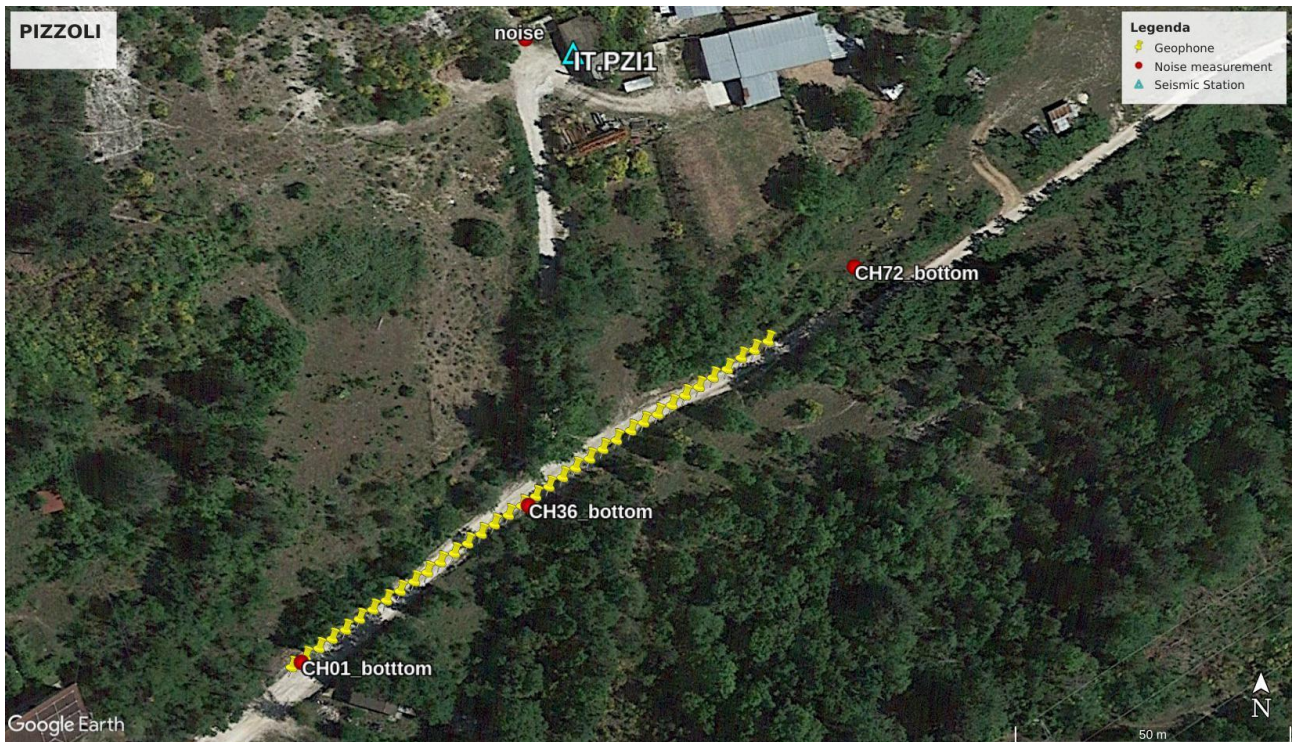
Figure 6. A zoomed view of the geophysical experiment close to ITPZI1. The linear array of vertical geophones (yellow markers) is also indicated as bottom MASW in this report. Image from Google Earth http://www.earth.google.com .
