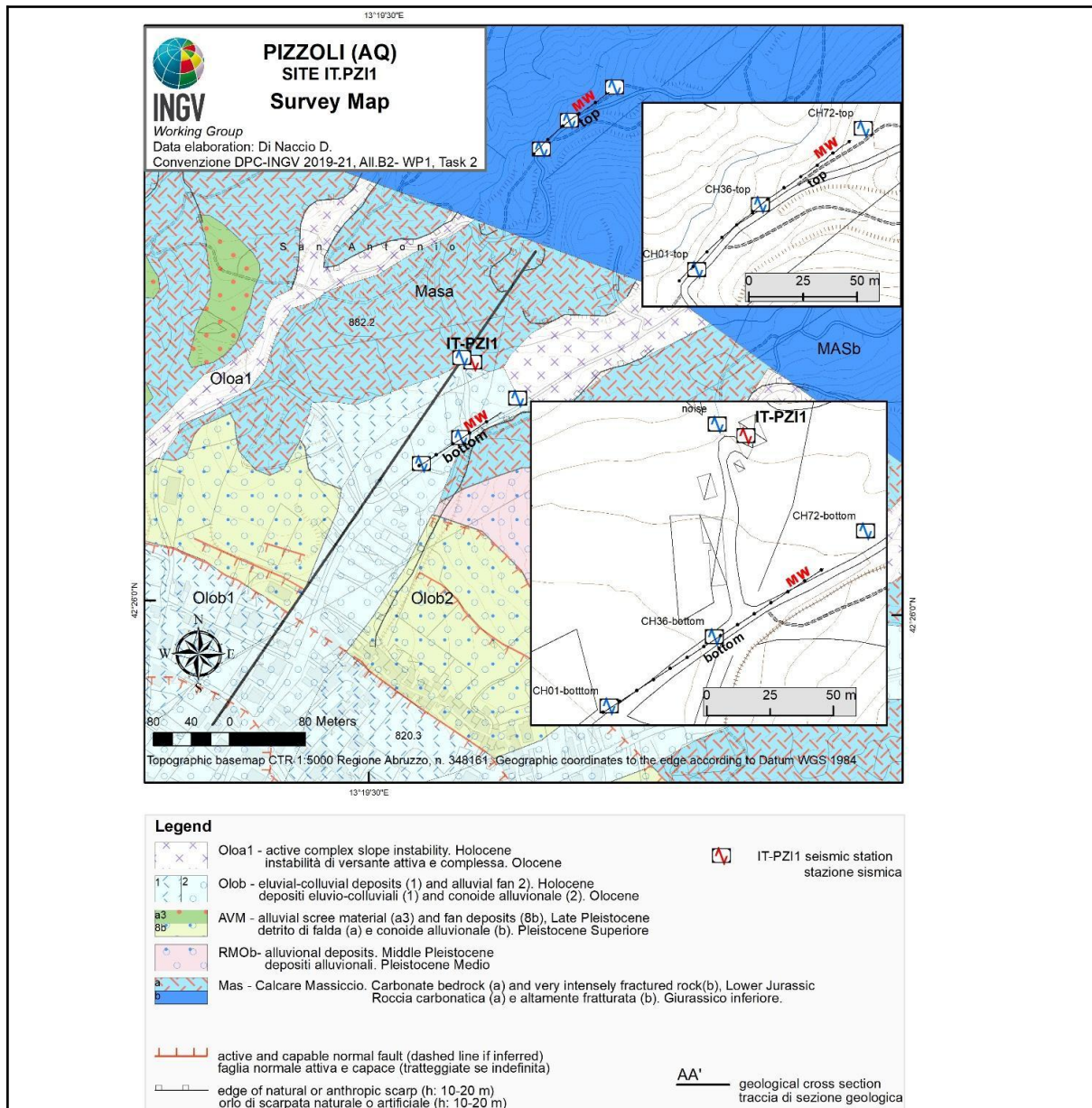
Figure 3. Map of the surveys in the surroundings of the IT.PZI1 seismic station. Scale 1:5.000. The maps at the right contain details of the geophysical survey conducted by the INGV Working Group for the seismic characterization of the site (Agreement DPC-INGV 2019-21, All. B2, WP1 - TASK 2). Refer also to part B “Vs profile” in this report.
