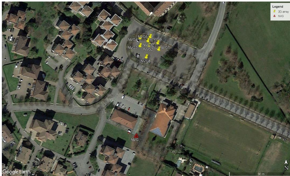
Figure 6: Map of the geophysical measurements performed at the IT.NVG site. The yellow place-markers indicate the geometry used for 2D array in passive configuration. The red triangle indicates the IT.NVG accelerometric station (image from Google Earth http://www.earth.google.com ).
