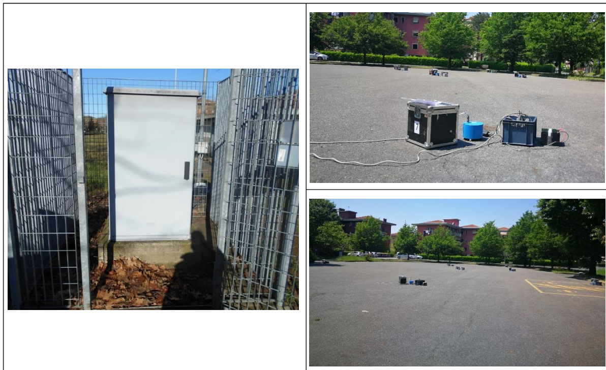
Figure 7: Left: IT.NVG accelerometric station installed in Novi Ligure (AL). Upper right: single station ambient noise measurement. Bottom right: 2D passive ambient noise array installed close to the IT.NVG station.
