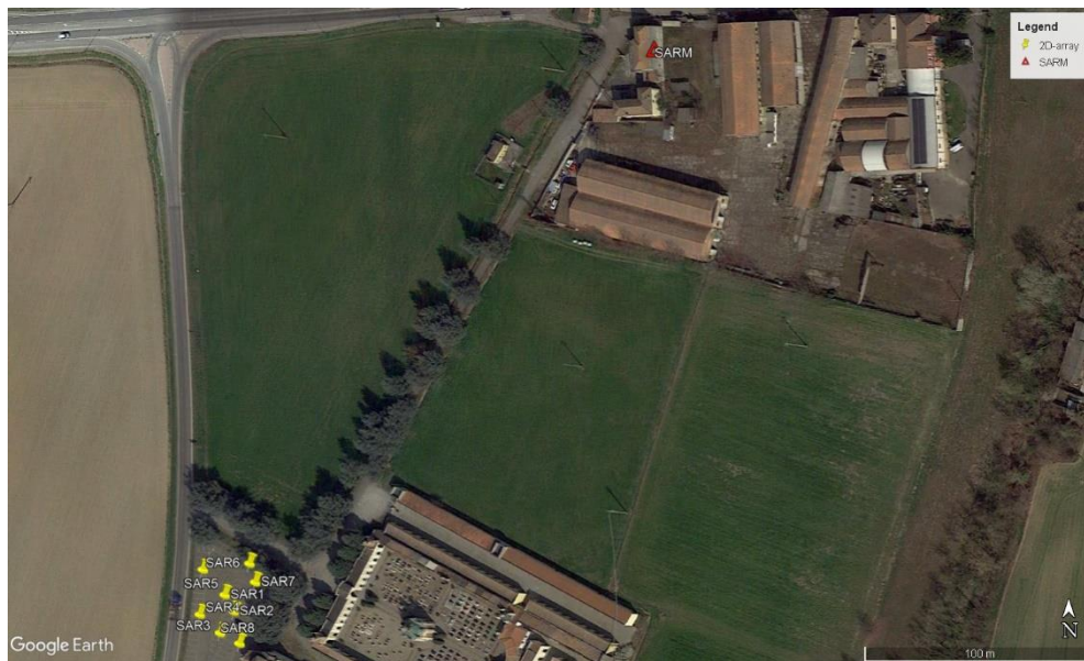
Figure 6: Map of the geophysical measurements performed at the IT.SARM site. The yellow place-markers indicate the geometry used for 2D array in passive configuration. The red triangle indicates the IT.SARM accelerometric station (image from Google Earth http://www.earth.google.com ).
