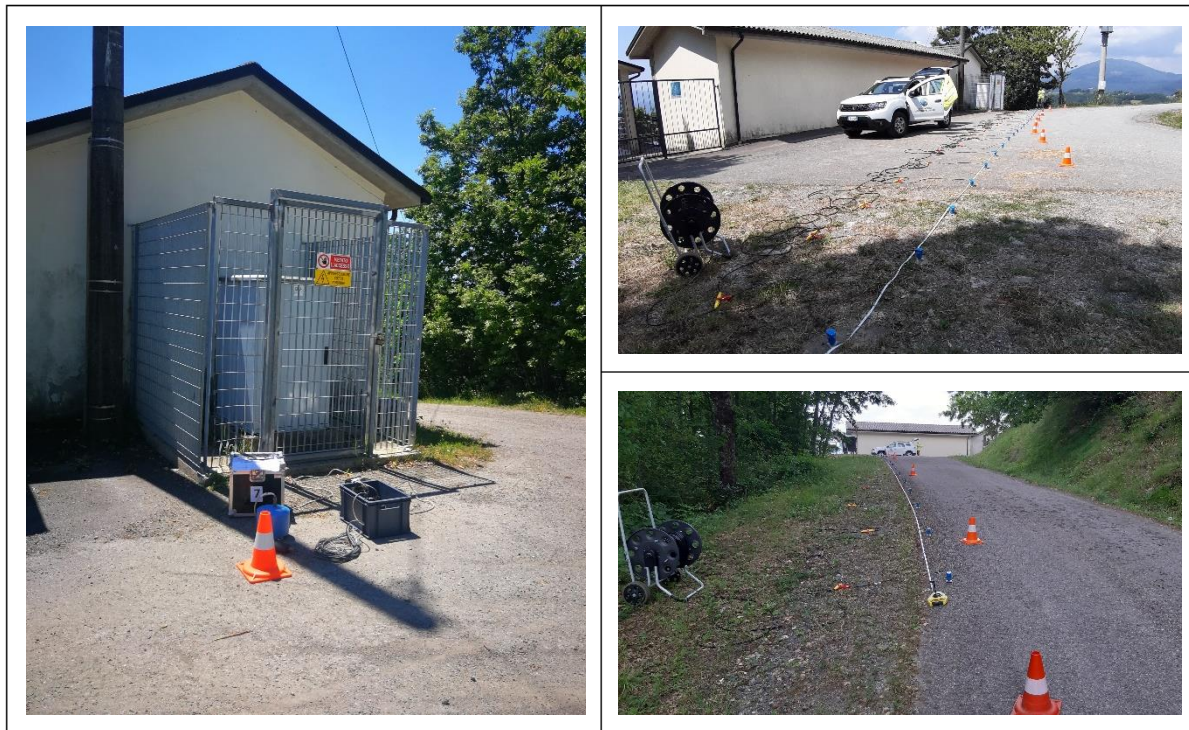
Figure 7: Left: IT.BVT accelerometric station installed in the municipality of Borgo Val di Taro (PR) and single station ambient noise measurement. Upper right: MASW acquisition line with 1 m receiver spacing. Bottom right: MASW acquisition line with 2 m receiver spacing.
