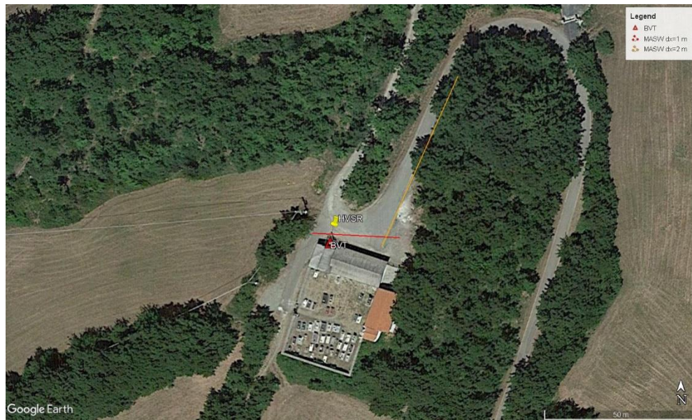
Figure 6: Map of the geophysical measurements performed at the IT.BVT site. The yellow place-marker indicates the single station ambient vibration measurement. The red line and the orange line indicate the lines of 24 geophones used for MASW, respectively with 1 m and 2 m receiver spacing. The red triangle indicates the IT.BVT accelerometric station (image from Google Earth http://www.earth.google.com ).
