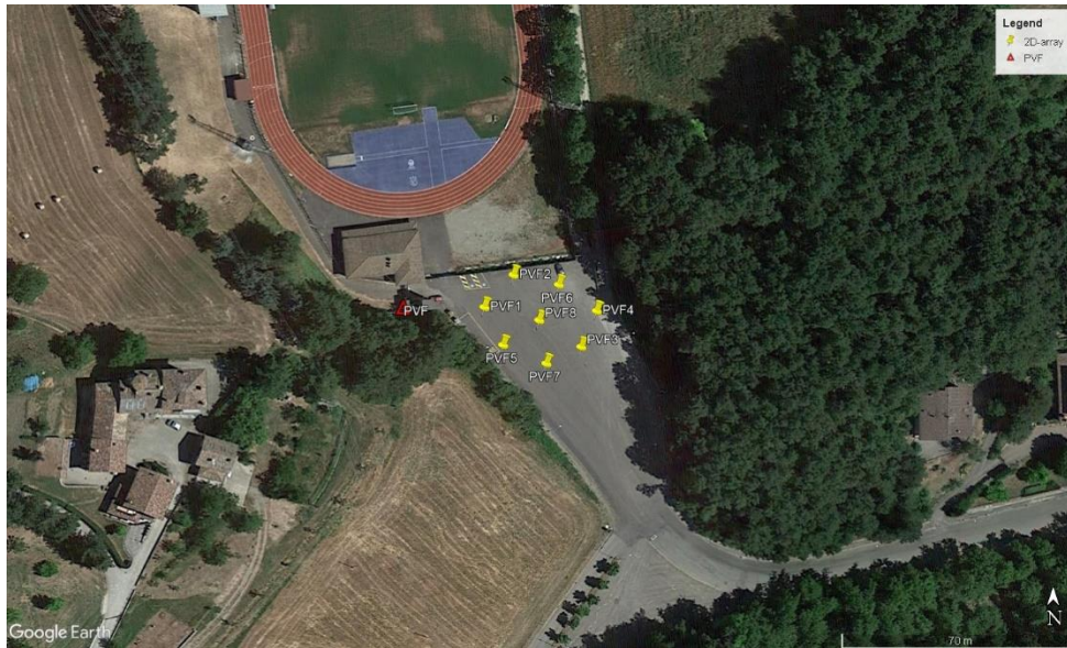
Figure 6: Map of the geophysical measurements performed at the IT.PVF site. The yellow place-markers indicate the geometry used for 2D array in passive configuration. The red triangle indicates the IT.PVF accelerometric station (image from Google Earth http://www.earth.google.com ).
