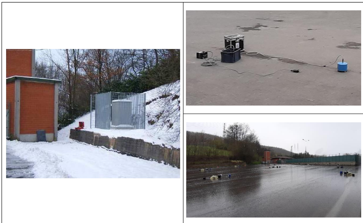
Figure 7: Left: IT.PVF accelerometric station installed in Pavullo nel Frignano (MO). Upper right: Single station ambient noise measurement. Bottom right: 2D passive ambient noise array installed close to the IT.PVF station.
