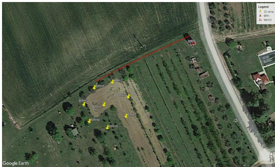
Figure 6: Map of the geophysical measurements performed at the IT.BRH site. The yellow place-markers indicate the geometry used for 2D array in passive configuration. The red line indicates the line of 24 geophones used for MASW. The red triangle indicates the IT.BRH accelerometric station (image from Google Earth http://www.earth.google.com ).
