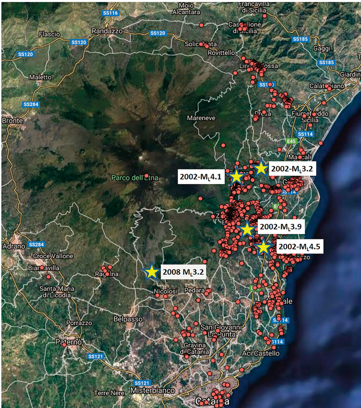
Figure 2. Map showing the location of the surveyed buildings (red dots) with AeDES forms collected after the 2002 and 2008 earthquakes in the Mt. Etna pilot area. The epicentres of the events selected for the analysis are marked by yellow stars.
