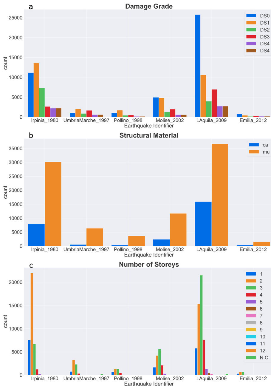
Fig. 12. Distribution of the different categories in the data collection with respect to the Earthquake Identifier. Panel a: Damage Grade; Panel b: Structural Material; Panel c: Number of Storeys. “N.C.” (Not compiled) implies that no information was available for that building in this category.
