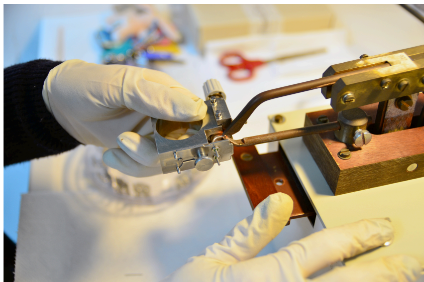
Figure 3. Preparation of the Re filaments for Sr and Nd isotope ratios measurements.
