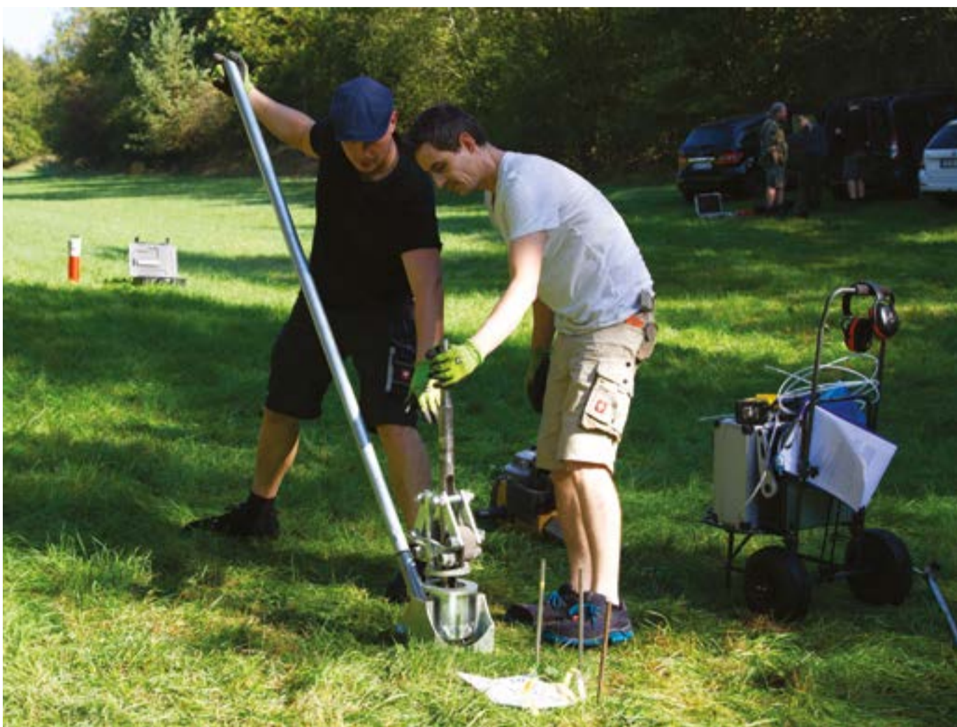
Soil-gas sampling drill, RIM 2018 exercise, Cetyne, Czech Republic. Source: Tore Tollefsen.
