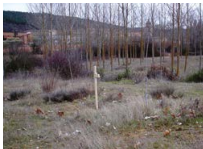
Outdoor radon detector placed 1 m above ground, Palencia province, Spain. Source: José-Luis Gutiérrez Villanueva.
