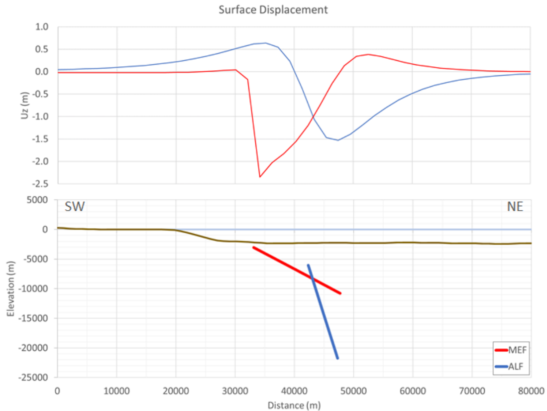
Figure 2. SW-NE profile, from southern Sicily into the Ionian offshore (see Figure 1 for location), crossing almost orthogonally the two earthquake ruptures (bottom). The seafloor (local surface) displacement in the middle of each earthquake rupture is projected onto the profile (top) for comparing the differences that, in this view, depend on dip and depth of the earthquake rupture, being all other parameters equal.
