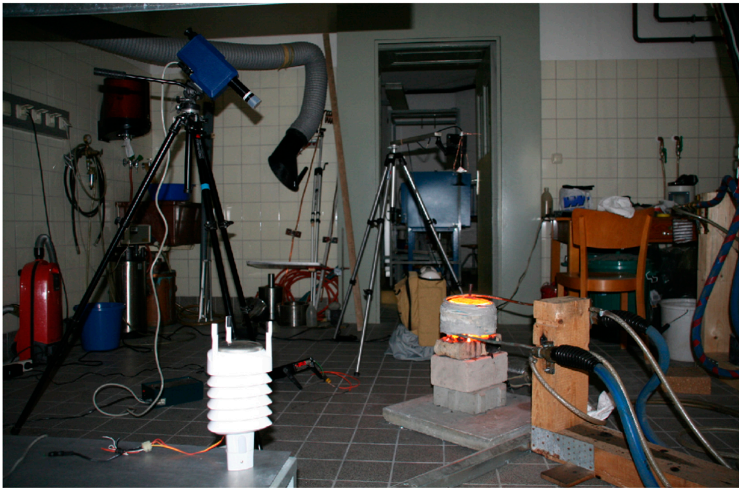
Figure 1. Experimental setup: basaltic rocks are melted in a steel crucible inductively heated using a radio frequency generator. In the background: the high spectral resolution portable spectrometer FieldSpec Pro for acquiring radiance spectra. To the left: thermocouple, pyrometer, and a thermal camera for providing punctual and spatially independent temperature measurements of the molten material. In the foreground: a portable meteo-station for continuously recording atmospheric ambient parameters to remove the effects of the atmosphere on acquired radiance spectra.
