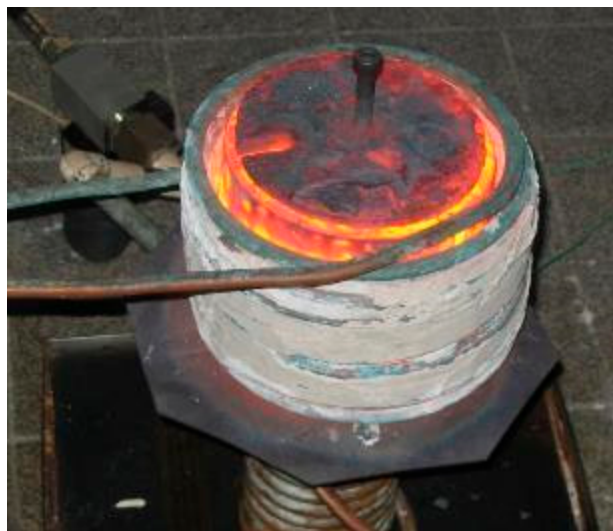
Figure 2. The steel crucible (10 cm inner diameter) with its lid during the melting phase of an experiment.
