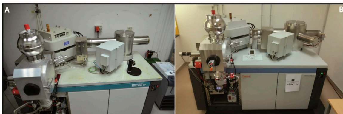
Figure 6. Photograph of the thermal ionization mass spectrometers: (A) the Triton TI at INGV, OV, and (B) the Triton Plus at DiSTAR.
