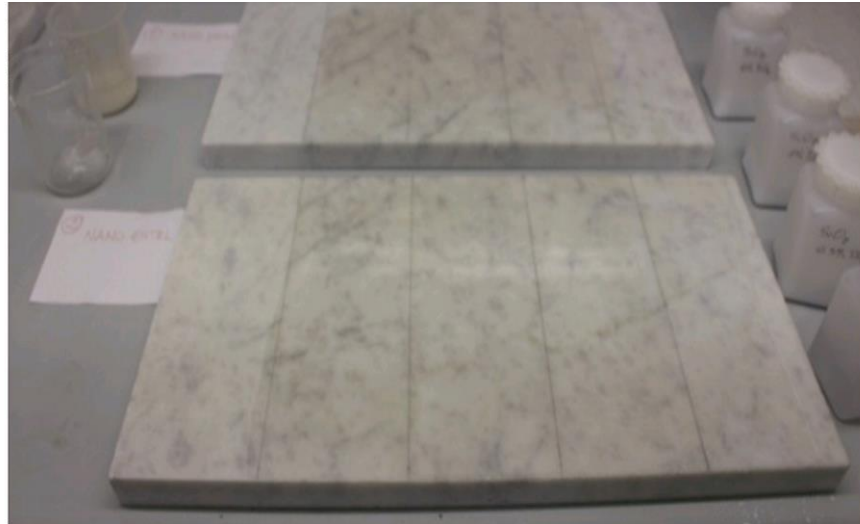
Figure 1. Laboratory marble samples with coatings blended with solutions of increased weight percentage concentration of titanium dioxide.
