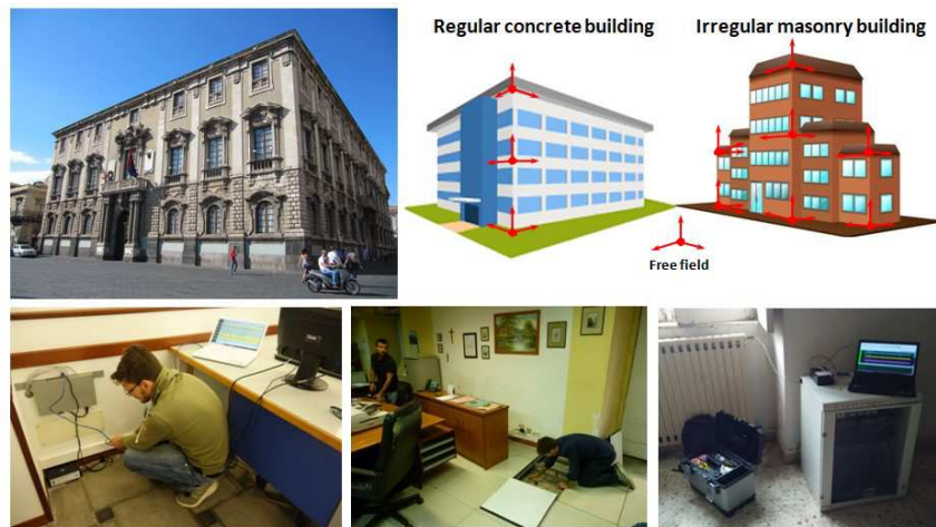
Fig. 3. Operation of installation and configuration of a monitoring station at the ground floor of the 18 th century “Elefanti Palace” located in the main square of Catania (Sicily Italy). Schemes for the sensors' distribution into edifices: a) minimum necessary requirements for a regular multi-storey building, and b) ideal extensive installations for irregular masonry buildings.
