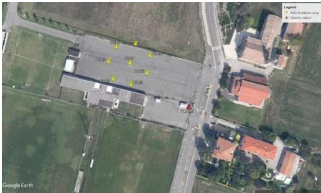
Figure 6: Map of the geophysical measurements performed at the IT.PAR site. The yellow placemarkers in circular geometry are the 8 stations of the 2D array in passive configuration. The red triangle indicates the IT.PAR accelerometric station (image from Google Earth http://www.earth.google.com ).
